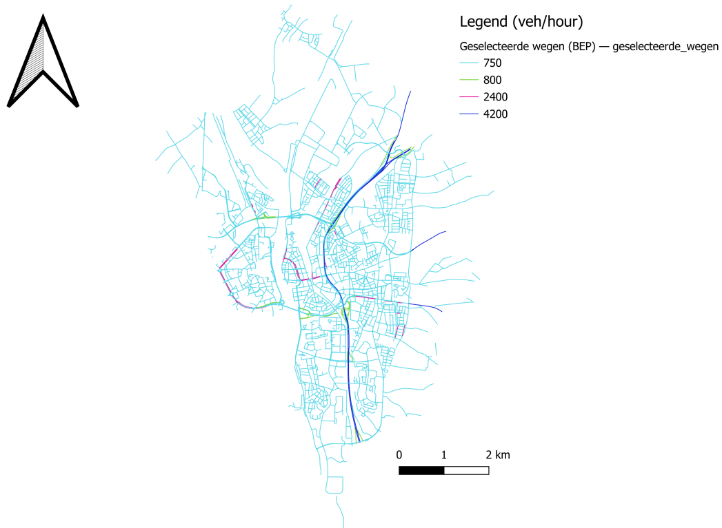
Figure 4.4: Estimated segment flow capacity ( Q_{\text{segment}} ) in veh/h per segment
