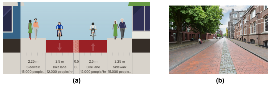
Figure 6.5: (a) Design 30 km/h roads without tram: Space for cyclists and pedestrians; (b) Example of a bicycle street: Ezelsveldlaan in Delft
