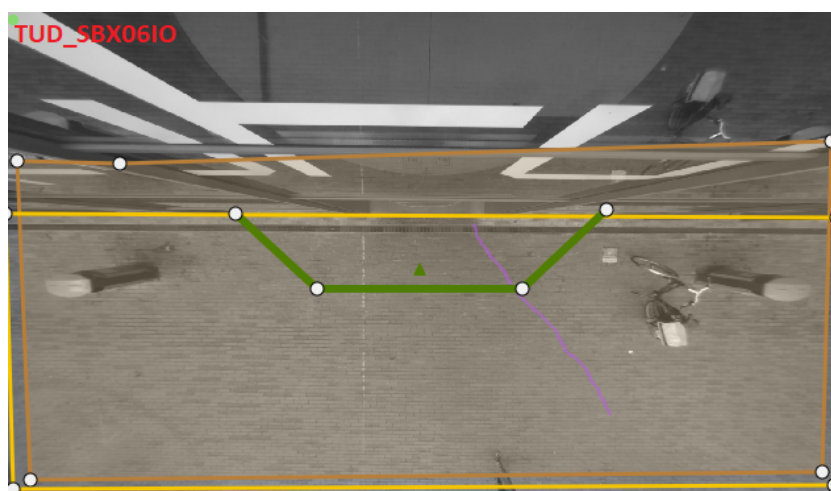
Figure 3.1: Detection area (orange) of the smart-sensor in front of the Industrial Design faculty (Daamen, 2023)
