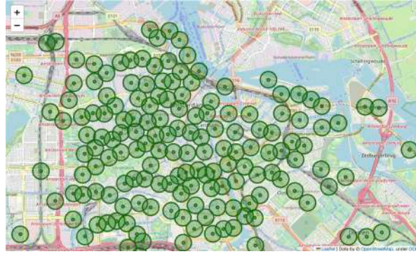
Figure 5.4: Coverage of the city with a radius of 225m, map from OpenStreetMap
