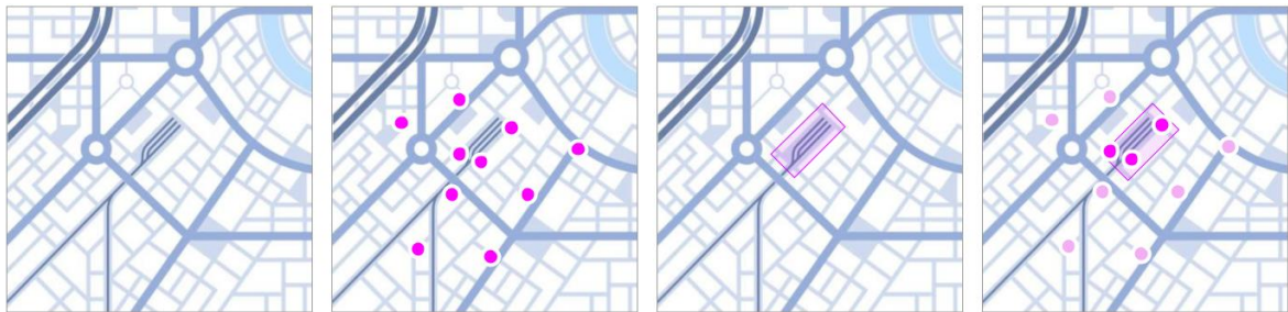
Figure 2.1: Method of last and first-mile calculation. Layers from left to right; The background map, start and end points, station zone, and calculation with n=3 trips inside the polygon.
