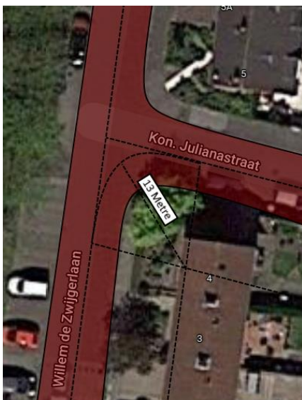
Figure 8 Approximation of the curve radii of the bends in the network, crossroad Koningin Julianastraat and Willem de Zwijgerlaan (Own work, dimensions and background image (Google Maps, 2021)).
