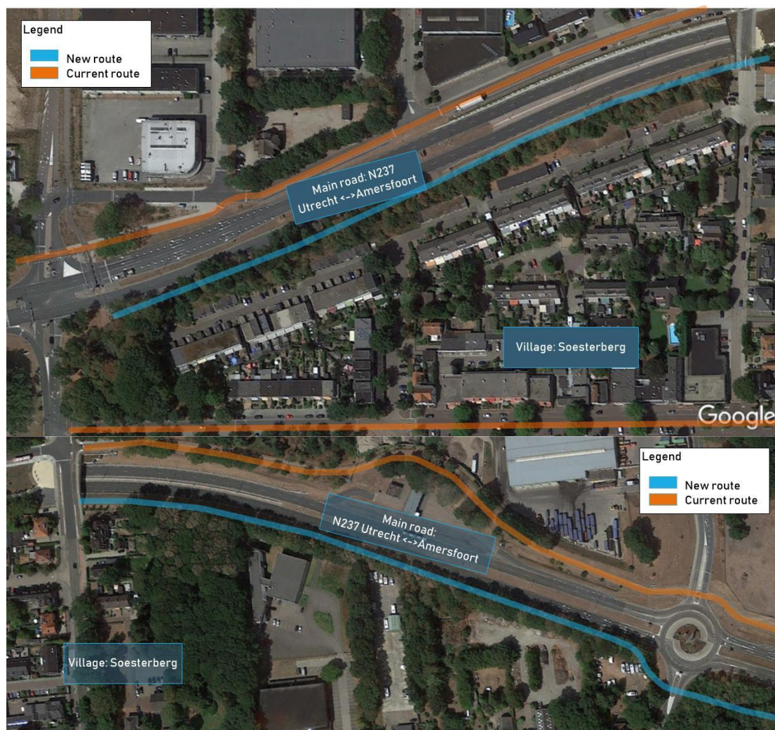
Figure 23, new bicycle path through Soesterberg. The bicycle path follows the N237, but stays at ground level. Above the western side of the tunnel, below the eastern side
